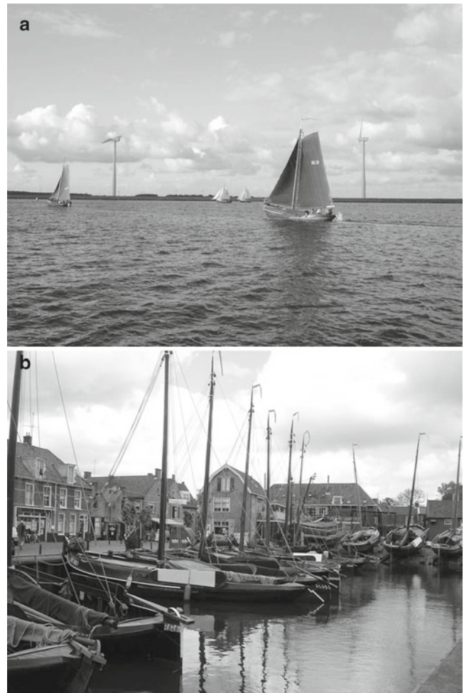
Fig. 4.3 (a) Traditional fishing boats (“Zuiderzee Botten”) still sail on IJssel Lake, but just for recreation. The boats are built for shallow water; they have side boards that are lowered when the winds are from the side to act as a keel. (b) Many of them are berthed in Spakenburg, an old Dutch eel-fishing village
